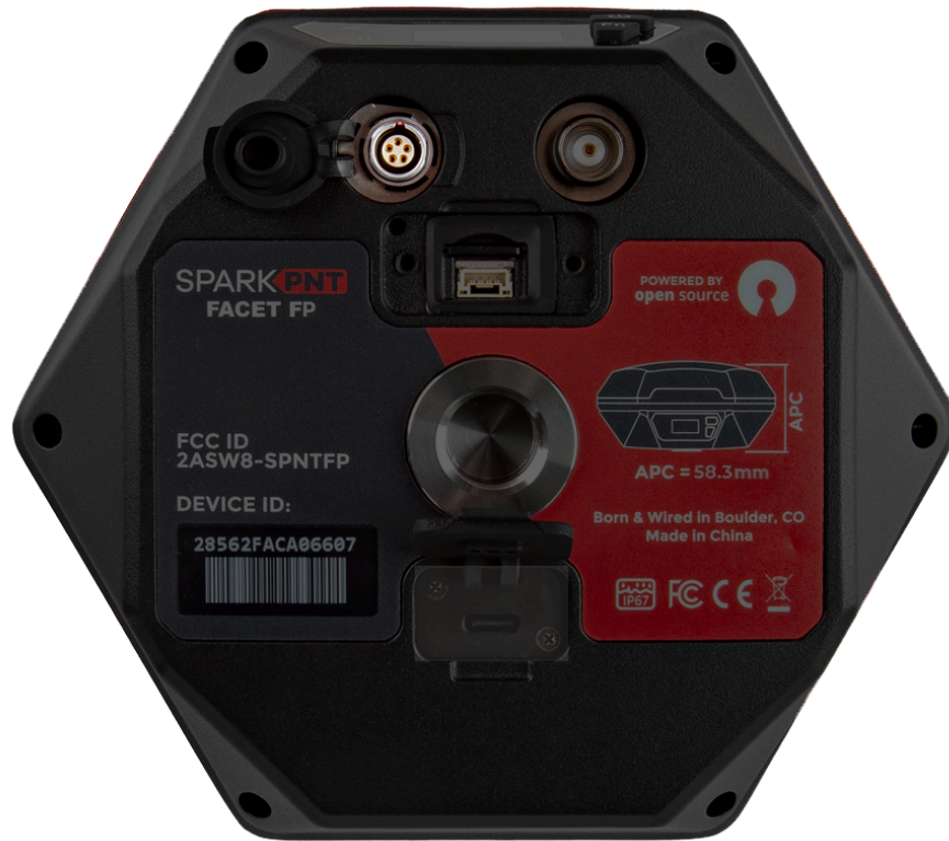
The Lemo-style connector on the bottom of the FPL.
