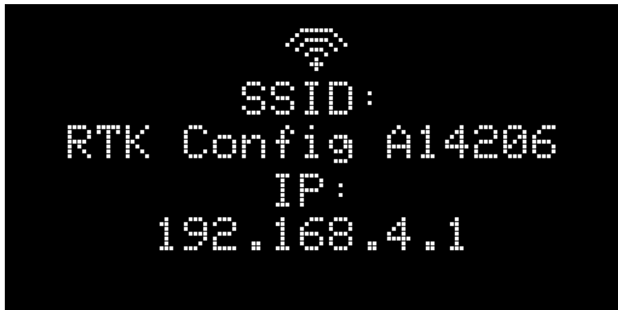
A device in Access Point configuration mode
