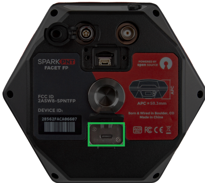
Users can access the USB-C port under the rubber cover on the bottom of the device.
