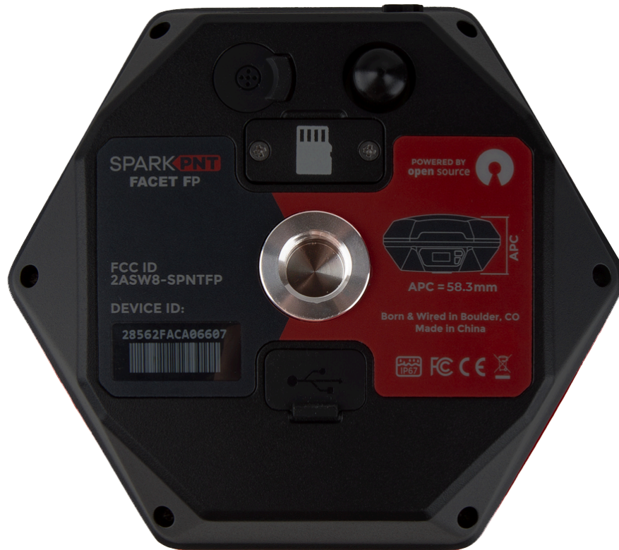
The 5/8"-11 TPI threaded insert on the base of the FPL.
