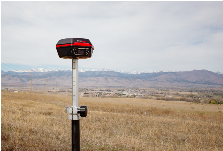
The SparkPNT FPL attached to a surveying pole.
