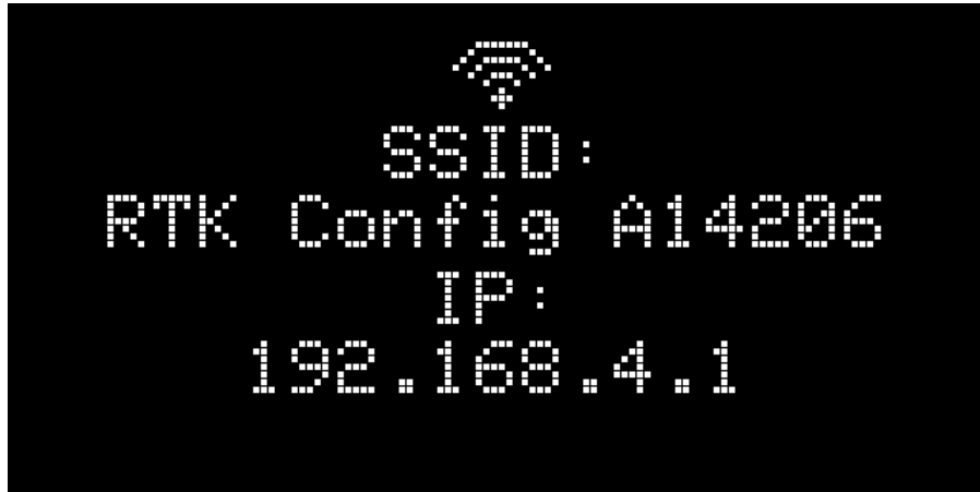
A device in Access Point configuration mode
