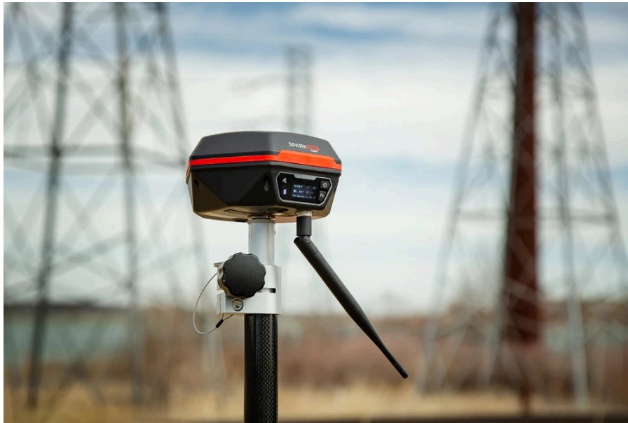
The SparkPNT FPM-T attached to a surveying pole.
