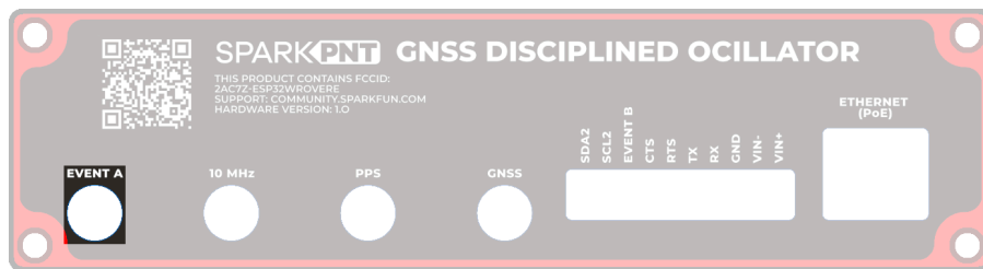
The SMA connector for the EventA input.
