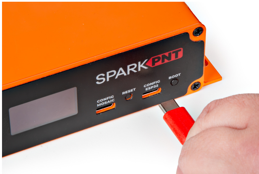
The GNSSDO(+) with USB-C cable being attached.
