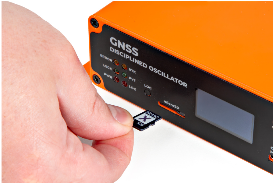
Inserting an SD card into the GNSSDO(+).
