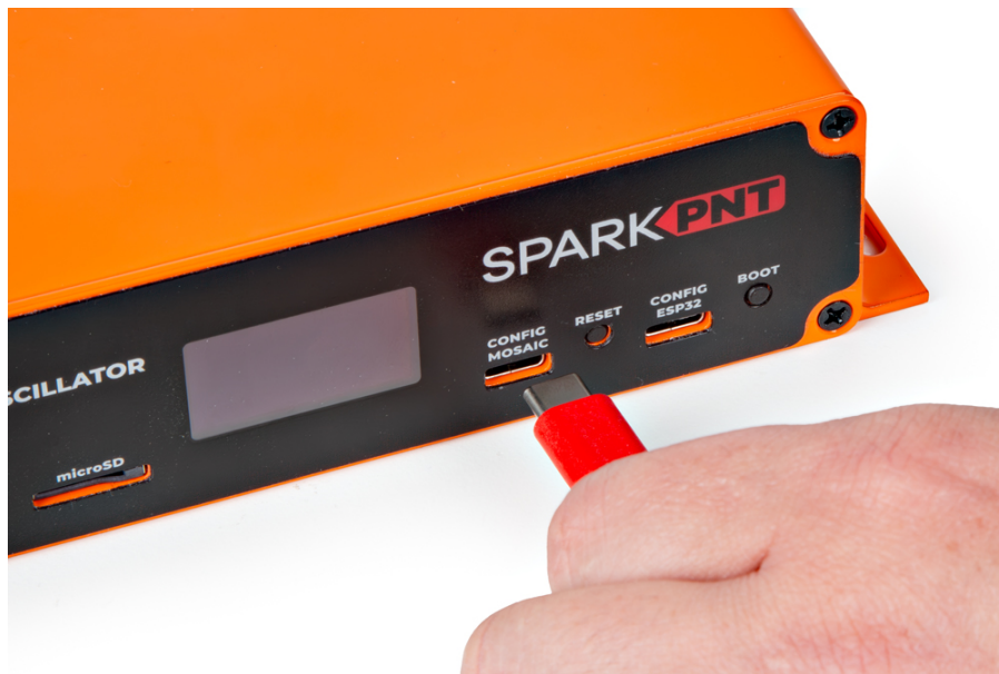
The GNSSDO(+) with USB-C cable being attached.
