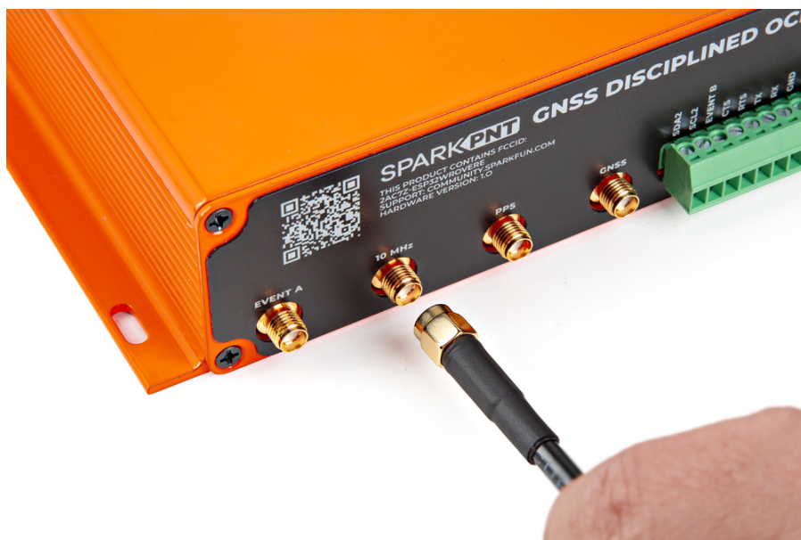
Attaching a cable to the 10MHz SMA connector on the GNSSDO(+).
