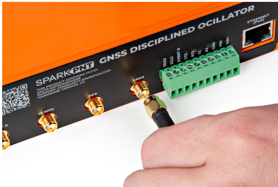
Attaching a TNC-SMA cable to the GNSS SMA connector on the GNSSDO(+).
