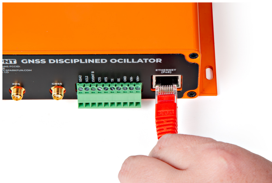
The GNSSDO(+) with ethernet cable being attached to the ETHERNET (PoE) jack.
