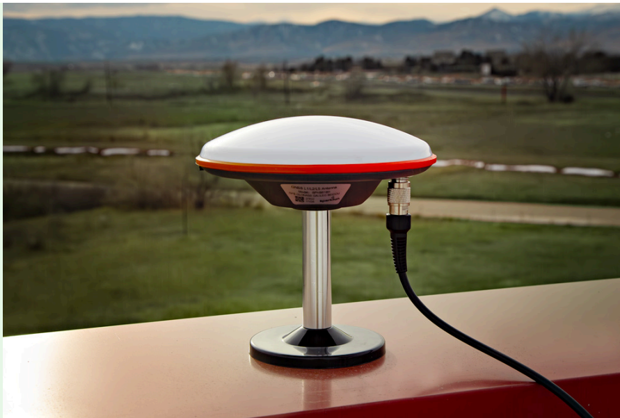
The tri-band GPS antenna, mounted outside with an unobstructed view of the sky.
