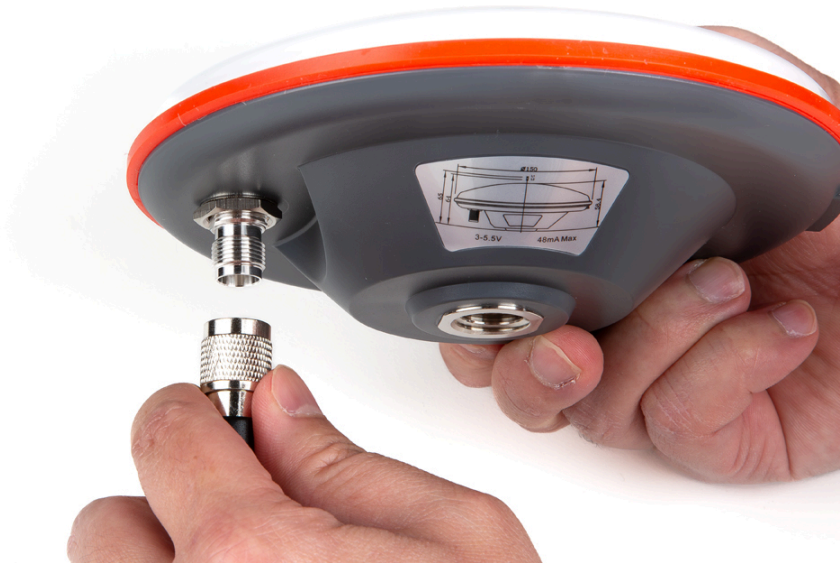
Attaching a tri-band GNSS antenna to the TNC-SMA cable.
