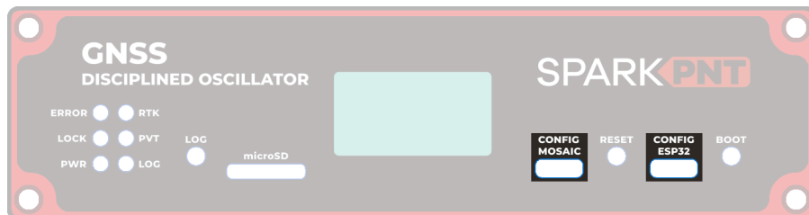
USB-C connections: mosaic-T (left) and ESP32 (right).
