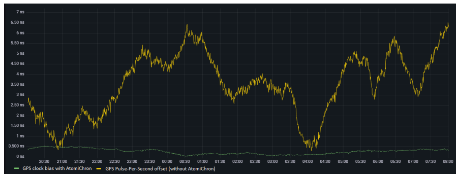
GPS clock bias with AtomiChron vs GPS Pulse-Per-Second offset (without AtomiChron).
